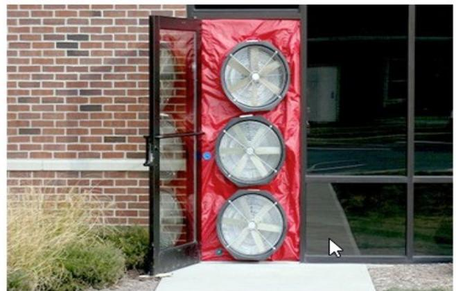
Thermal imaging and blower door testing are tools used for commissioning of the building enclosure.
