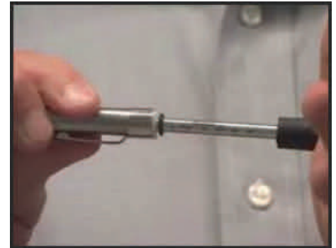
Pressure gages similar to the above are often used to measure opening force.
